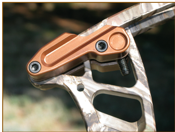
The bow's unique VX Limb Pockets lock the limb butts in place. Two cross-pocket clamping bolts are used to draw the right and left sides of the pockets together like a vise.
