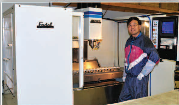
Liberty Archery's Tony Liu readies a Fadal CNC machine in the company's Santa Clara, California, facility for another run of limb pockets for the Liberty I bow.
