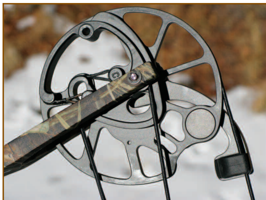
This is the lower drive cam on the Mission Journey. It's a state-of-the-art one-cam that draws smoothly and is wonderfully fast.
