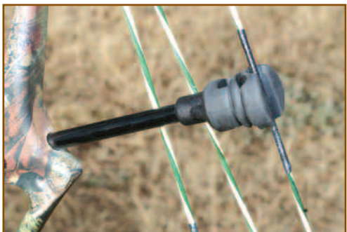
Hoyt's StealthShot String Suppression System, which projects out of the back of the Katera below the grip, momentarily captures the forward-moving bowstring in a LimbSaver Navcom bumper, instantly stopping and dampening the bowstring.
