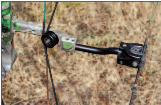
The new BowTech Roller Guard/ShortStop String Suppressor captures and tensions the bow's cables, as well as catching, centering and dampening the bow's bowstring.
